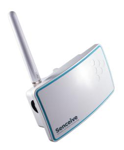
The Digital Interface Node is a robust IP66/IP67 rated digital data logger that transforms your data collection from manual to automated sampling. This wireless digital data logger is compatible with a large variety of sensors that carry a digital output and enables a simple connection to the Senceive back-end & front-end platforms. Interact and manage your data online and change reporting times and thresholds remotely.
